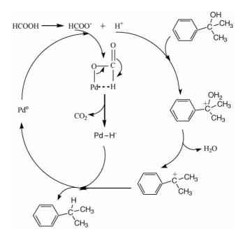
Scheme 1. Mechanism of transfer hydrogenolysis of 2-phenyl-2-propanol over Pd/C with formic acid.
