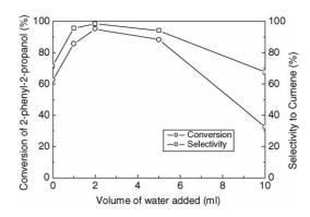
Fig. 2. Effect of water content in ethanol solvent on the transfer hydrogenolysis with formic acid over Pd/C catalyst at 80 °C for 4 h.
