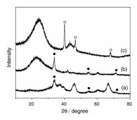
Fig. 1. XRD patterns of the catalysts untreated of Pd/Al<sub>2</sub>O<sub>3</sub> (a), Pd/MCM-41 (b) and Pd/C (c).  $\bigcirc$ , Pd<sup>0</sup>;  $\bigcirc$ , PdO.
